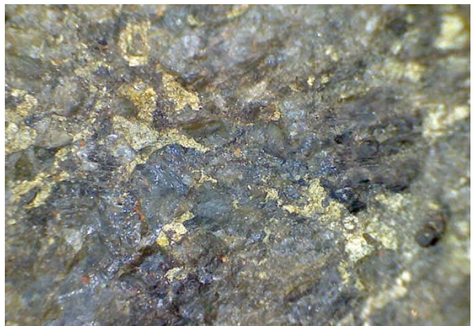
FRR013, 81-82m, disseminated pyrite and chalcopyrite mineralisation, copper grade 0.61%. 25X magnification.
